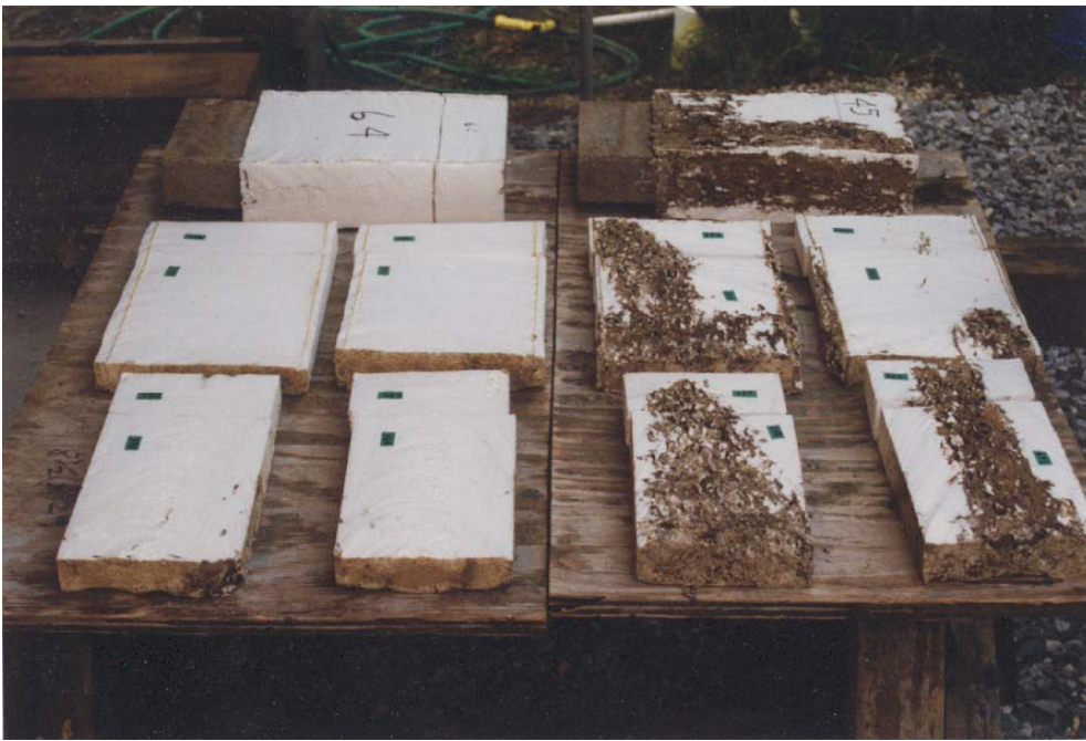
#64 TEST FIXTURE - ThermaFoam R-Control with Perform Guard and R-Control Do-All-Ply.
