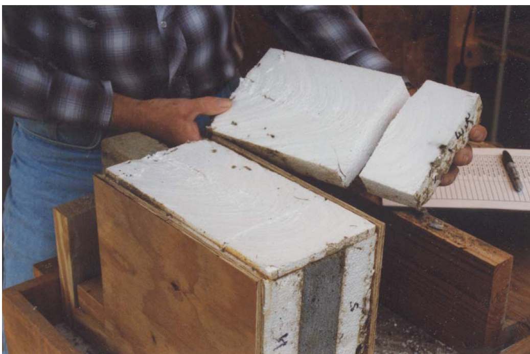
#64 TEST FIXTURE - Close-up shows slight termite damage.
