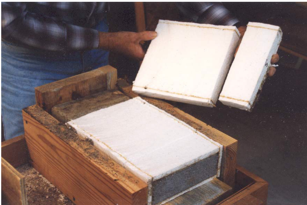
#64 TEST FIXTURE - Close-up shows no termite damage.
