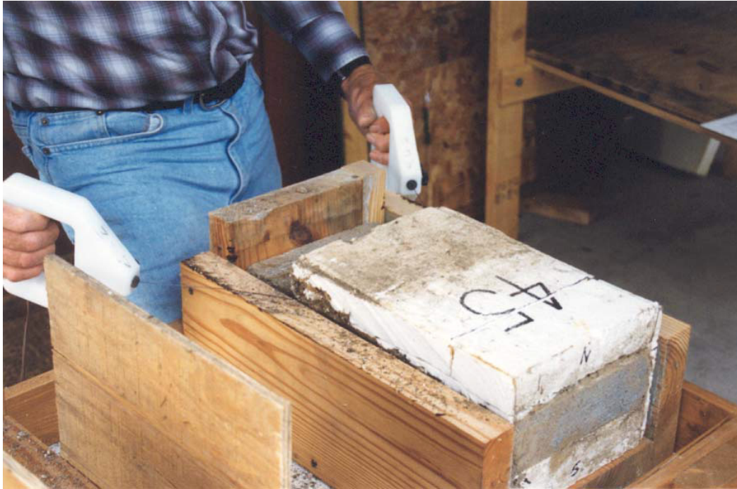
#45 TEST FIXTURE - Examination of of non-treated EPS after 3 years exposure. Highland Site, Mississippi.
